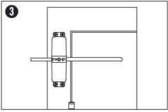
While holding center of closer, attach arm into threaded hole closest to the door.
