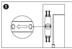
Attach closer to hinge side of door with arrow facing away from door.
