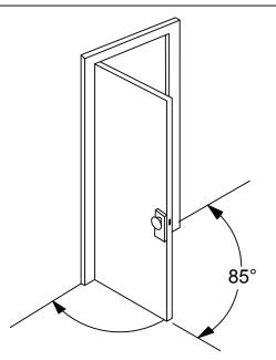
This door closer has a built in, non-adjustable hold open feature. If the door is opened beyond 85 degrees, the door will remain open until it is pulled back to less than 85 degrees, then it will close automatically.
