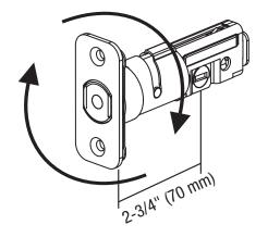
Use the following steps to prepare your door for a new installation, or to verify dimensions for a replacement installation.
