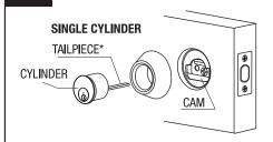
\*Keep cylinder tailpiece <u>HORIZONTAL</u> while inserting it into cam slot.
