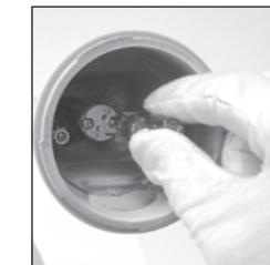
Remove the old bulb by gently pulling the bulb straight out of the socket. Insert new bulb by aligning the bulb prongs with the socket and gently pushing the bulb straight in until it is properly seated.
