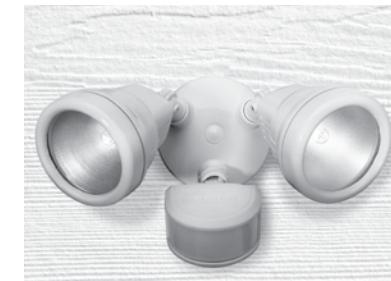
Position lamp holders downward at a minimum 45° and away from fixture housing a minimum of 2 inches. Aim the motion sensor at the center of the desired detection area. **Bulbs are pre-installed - See back page for replacement instructions.**
