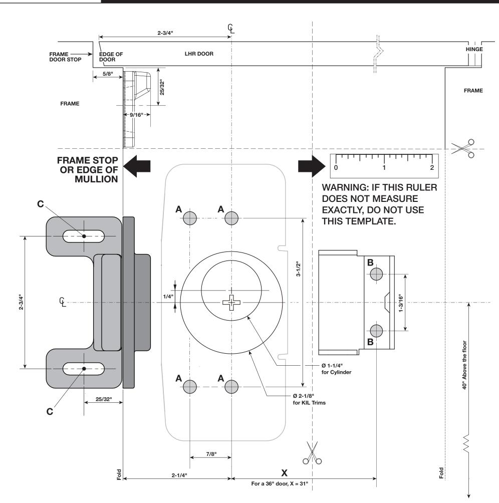
NOTE: If using BC40011 or BC40012 trim, use the supplied template with those devices and place on the outside face of the door.
