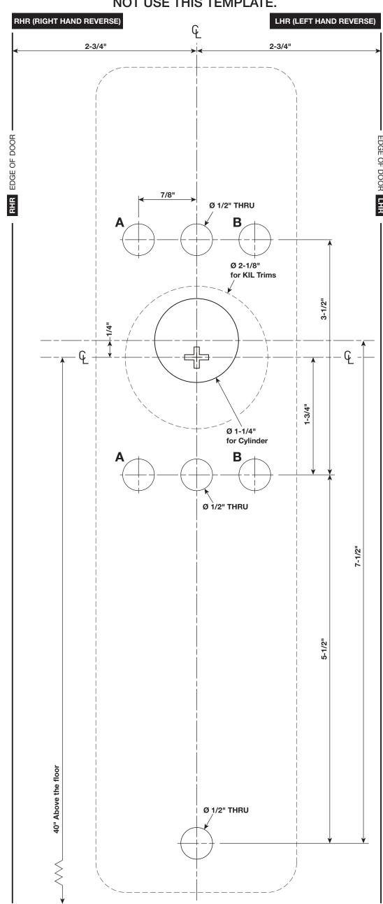
The BC40011 Pull Handle is only to be used with the BC40010 Rim Exit Device. The cylinder, collar, cylinder mounting plate and S8 cylinder mounting screws are included with BC40010.
